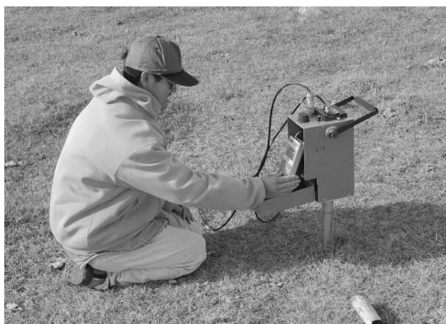
Xuejun Dong takes soil moisture readings using a neutron moisture meter.
